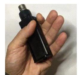
The PWL is a Phantom 48V mic powering, running on a single AA battery.
